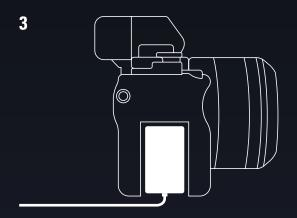
Use an AC Adapter - Most cameras cannot operate and charge at the same time. An AC adapter or "dummy battery" must be used to trick the camera into thinking it is running on battery power indefinitely.
