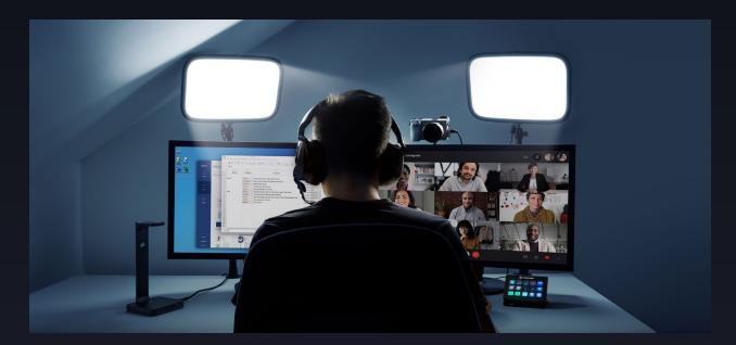
When using more than one Key Light, position them on either side of your desk, aimed at your face at a 45-degree angle. This is the best way to properly illuminate a green screen or wall that is behind you, and eliminate shadows that would be created by a single light source. Key Light features adjustable brightness and color temperature, so you can set ideal lighting conditions for your workspace.
