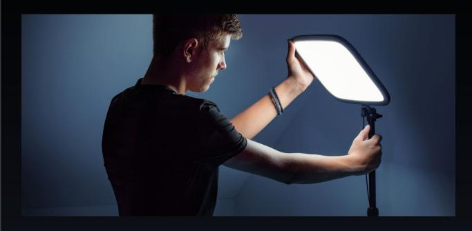
When using a single Key Light as an additional light source, you can position it alongside your other light source to eliminate shadows on your face. If Key Light is your primary light source, position it directly in front of you, just above your eyeline, angled downward at approximately 30 degrees. This lighting method creates a dramatic and professional look.
