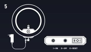
Connect the power supply to Ring Light and plug it into a wall outlet.
