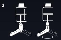
Turn the twist lock to adjust the height of Master Mount S.
